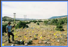
Maureen Boyle stands holding the Thales Promark 3 GPS rover. The unit was held above each stone in the circle as information was sent from the rover to the base station.
