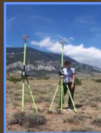
The two Thales Promark 3 GPS units used by students to take UTM coordinate data for each stone circle.
